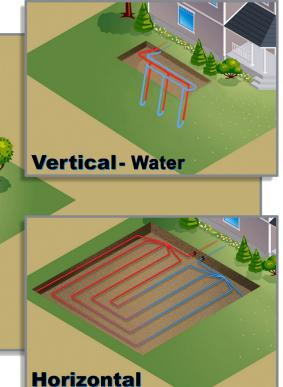
Ground Loop Design: Designing an efficient ground loop system requires four critical aspects: loop layout, ground loop material, amount of loop being installed, and the loop fluid. Although each one of these is important, it all begins with deciding which loop layout makes the most sense for you. The loop layout can be either a horizontal ground loop or a vertical ground loop (the ground loop material and the loop fluid will be addressed later in the article).
